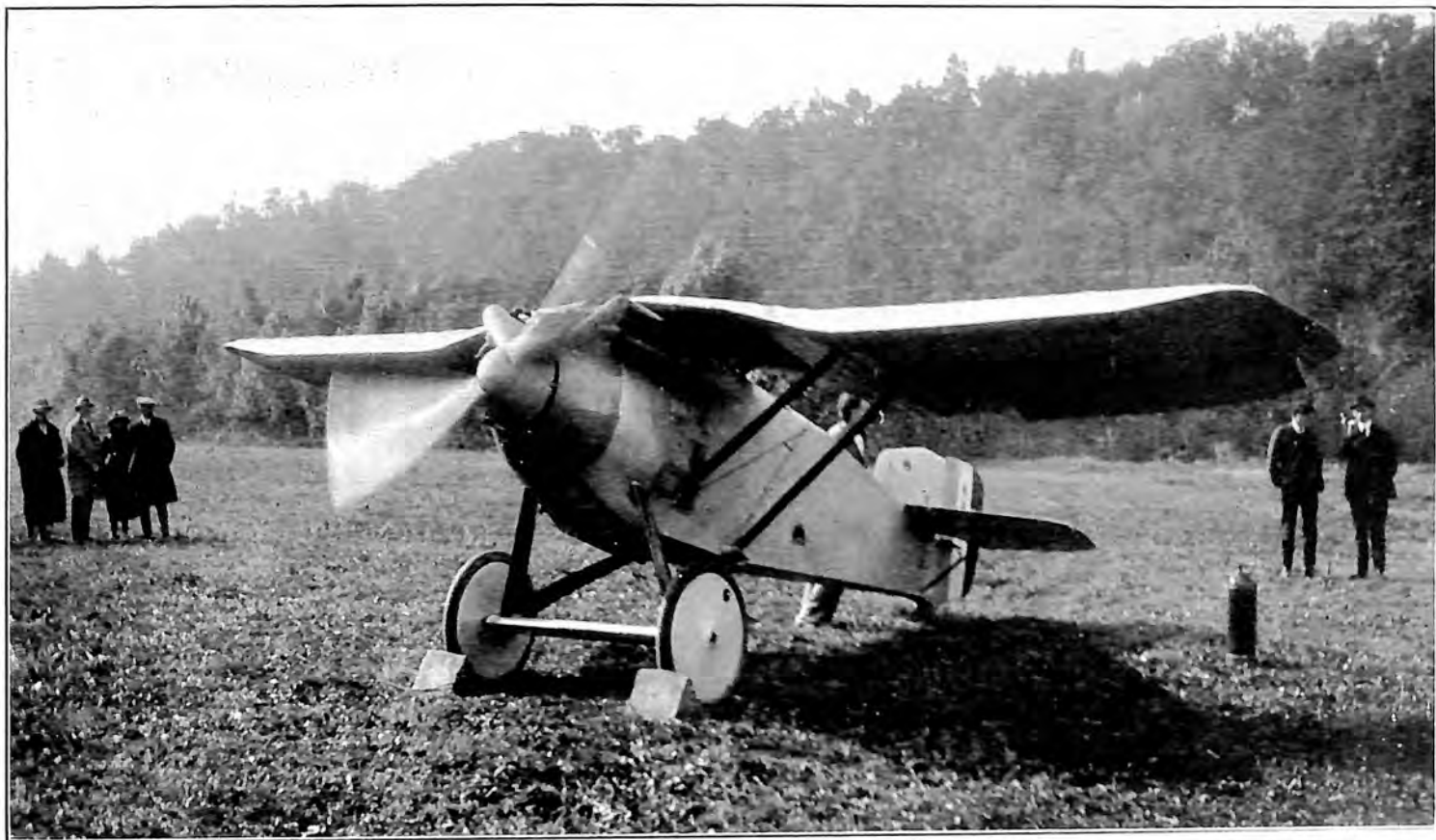
Thomas-Morse M. B.-7 type of fighting monoplane, 400 h.p. Wright H.-3 engine. Developed for air service and contender in 1922 Pulitzer race.
