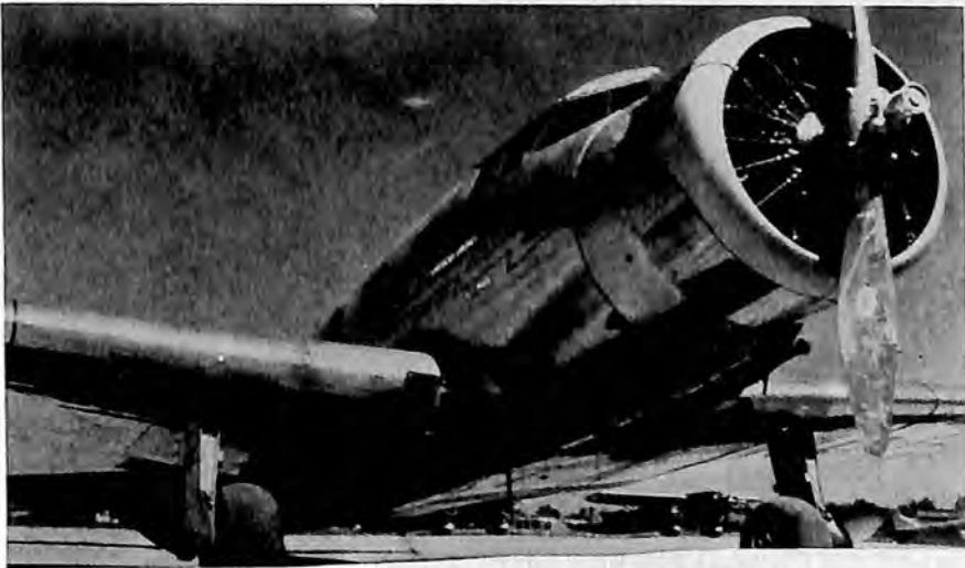
AMERICAN AIRLINES VULTEE TRANSPORT Showing Cyclone engine and Hamilton Standard propeller.
