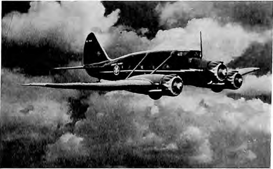
One of the Model A passenger ships with three Lycoming engines and Smith controllable pitch propellers in service on the short routes of American Airlines.
