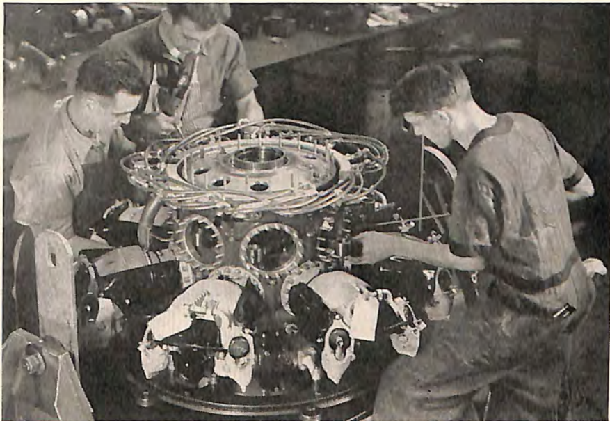
INSTALLING TWIN WASP CYLINDERS
