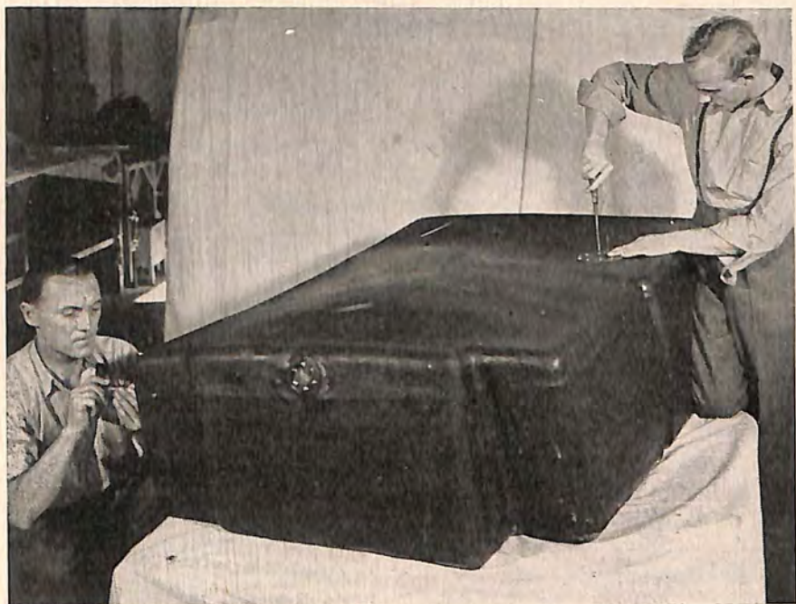
FIRESTONE BULLET-SEALING FUEL TANK
