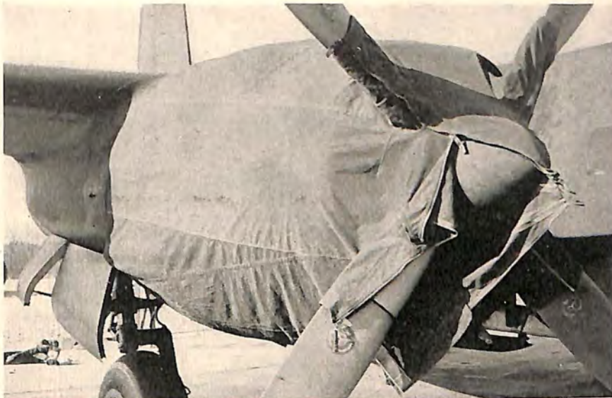
CROWN FASTENER ZIPPER COVER On an engine of the Martin B-26 bomber.
