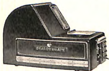
SHADOWGRAPH, Type A, an electrically operated scale for piston selection and precision.
