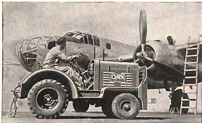
"Clarks" maneuver planes in hangars and on the flight ramps at every U. S. Army Airfield.
