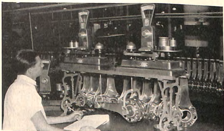
An efficient connecting rod selection operation in the Wright Aeronautical Corporation, Paterson, N. J. Tolerance is to 0.03 lb. of a predetermined standard weight.
