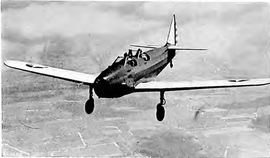
FAIRCHILD AIR CORPS TRAINER IN FLIGHT The PT-19, powered with a Ranger or a Warner engine.
