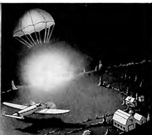
Bracket of four 1½-Minute (electrically operated) Parachute Flares, each of which will develop more than 110,000 candlepower.
