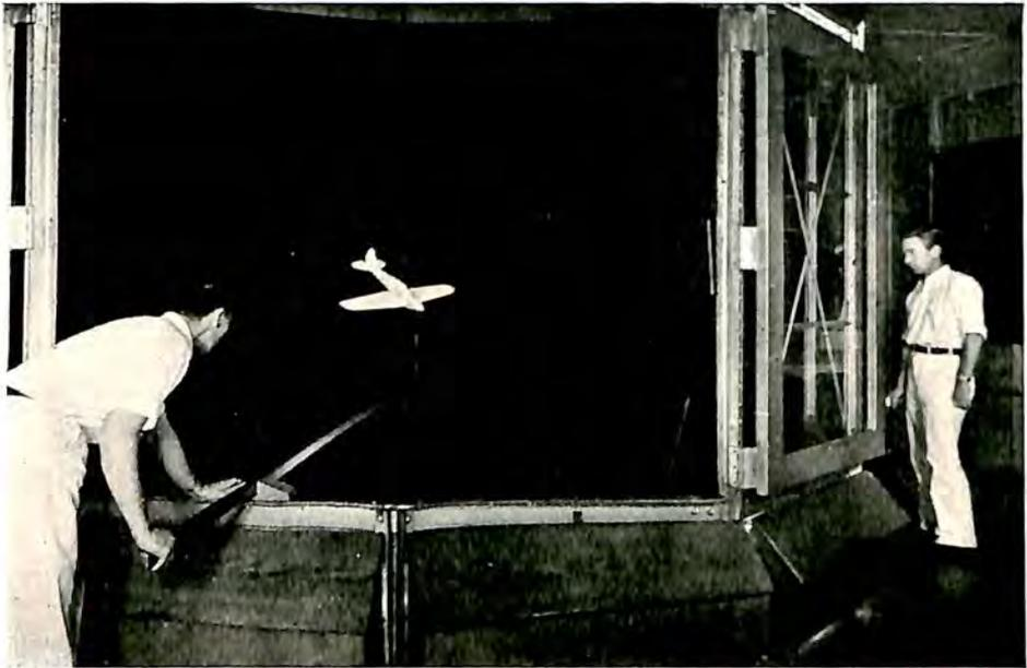
THE FREE-SPINNING WIND TUNNEL
