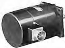
Light-weight precision-balance G-E aircraft motors are made from 1/200 to 7 hp. Speeds range from 1750 to 7500 rpm. Series-, compound-, or shunt-wound, they meet various applications. Standard Air Corps flange mounting styles 2 to 4.
