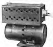
Aircraft high frequency motor alternator set for operating radio equipment.
