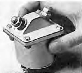
Dynamotor contactor—will handle an inrush of 500 amperes at 32 volts. It operates on either 12 or 24 volts, d-c. Provides one single-pole normally open contact; has a 50-ampere rating based on NEMA 8-hour test.
