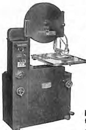
**CAST IRON** and a variety of sawing can be accomplished in jig-time with the Type GV-1 (right). Available in any 3:1 speed variation from 100:300 to 1000:3000 blade feet per minute.
