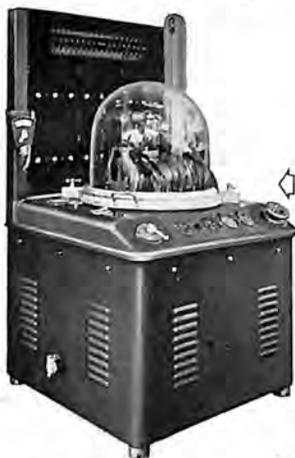
Magneto Test Stand, for testing airplane magnetos at speeds from 50 to 6500 r.p.m. and at various conditions of heat, humidity and altitude. ◇
