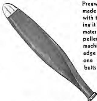
Pregwood is a special grade of Formica made by impregnating thin plywood with thermosetting resins and vulcanizing it into a strong, hard, homogeneous material, from blocks of which propeller blades and propeller parts are machined. The material is also used for edge strips to hold fastenings, where one section of a plywood structure butts up against the next.
