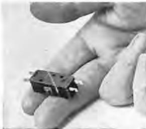
Although it's small, the G-F Switchette has double-break contact construction. It weighs only  $\frac{1}{3}$  ounce and measures  $1\frac{3}{4}$  by  $\frac{1}{2}$  by  $\frac{1}{2}$  in. Made in single or two-circuit form. One contact normally open—one closed; or vice versa.
