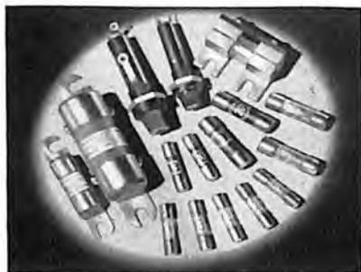
With Littelfuse Locked Cap Assembly, caps can not be loosened. Markings not lost. "Gooseneck" non-crystallizing element, absorbs contraction, expansion. Element twisted at 90°, braces for severest vibration. Littelfuse superiorities insure Dependability—longest life.
