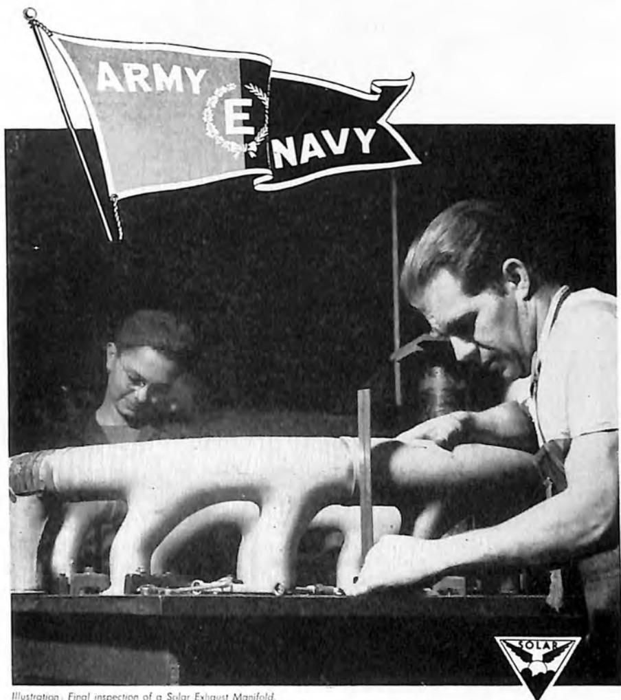
Illustration: Final inspection of a Solar Exhaust Manifold.
