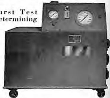
◇ Denison electric motor driven HydroOILic Test Stand for testing aircraft hydraulic systems using up to 1500 pound pressures. A similar unit, for 3,000 pound pressures, is also available.
