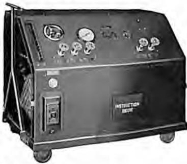
Denison Burst Test Stand for determining burst pressures of devices in hydraulic systems. ◇
