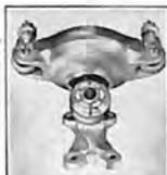
Primarily, the Type RS-40 Dynafocal Suspension was developed for use with the Wright 18 Cylinder Cyclone Engine. It was designed with the thought of including the more desirable features of the earlier link type and flexible pedestal type suspension, and in addition, provide effective snubbing and damping means through the use of three ball joints and a rubber snubbing ring. Write for data.
