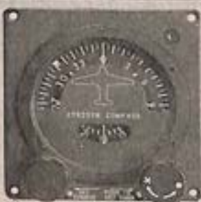
Sperry Gyrosyn Compass Model C-1, now in production. Rotating Dial Type illustrated—available also with Pointer Indicator.
